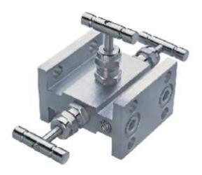
**MIC** 3 way valve manifolds are mainly used in differential pressure transmitters and static instrument applications such as pressure switches, pressure transmitter and manometers. It has two process isolation valves and one equalization valve to equalize the two sides. Process and instrument sides are both on 54 mm centers to correspond with transmitter connection.
